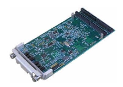
THE PMC SATA CONTROLLER is a PMC Mezzanine card with a dual-channel 64-bit PCI/PCI-X SATA 3 controller with 2 SATA connectors via front panel.
