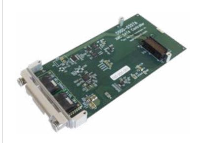
THE XMC SATA CONTROLLER is an XMC Mezzanine card with a dual-channel PCIe Gen 2x2 SATA 3 controller with 2 SATA connectors via front panel.
