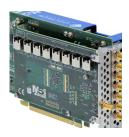
The Star-Hub is an additional module allowing the phase stable synchronization of up to 8 boards of one series and with same speed grade in one system. Independent of the number of boards there is no phase delay between all channels. The Star-Hub distributes trigger and clock information between all boards to ensure all connected boards are running with the same clock and trigger. All trigger
