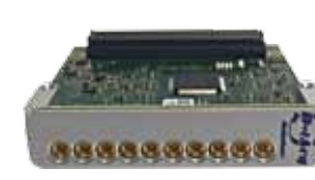
ACQ480FMC (80MHz 14bit 8ch A/D)
