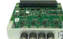
AO420FMC (1MHz 20bit 4ch D/A)
